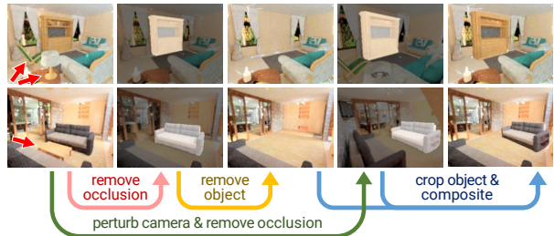
Figure 5: Rendering pipeline. Given an indoor scene and a candidate object, we remove occluding objects to create an occlusion-free scenario, which we do the same at another perturbed camera pose. We further remove the object to create a training sample pair with mismatched perspectives.
