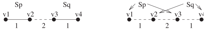
Fig. 3. An example collision when vertices with positive gains migrated simultaneously result in an increase in cost.
