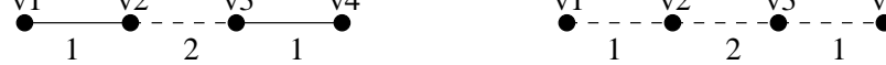
Figure 4: An example collision when vertices with positive gains migrated simultaneously result in an increase in cost.
