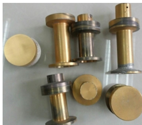
Figure 10 Test pieces with Au coating on the sealing face
