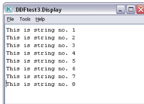
FIGURE 0.20: THE OUTPUT OF THE EXAMPLE WORKFLOW ONCE A REQUIREDFIRINGSPERITERATION PARAMETER HAS BEEN ADDED TO THE BOOLEANSWITCH ACTOR.
