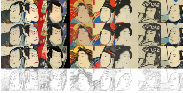
Figure 16: Comparison of conditional and the unconditional colorization method. The former uses style reference images while the latter does not. Four rows are the ground truth color image, conditional colorization, unconditional colorization, and line art sketches, respectively.
