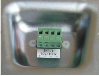
Figure 5: Plugging and Securing the Cable
