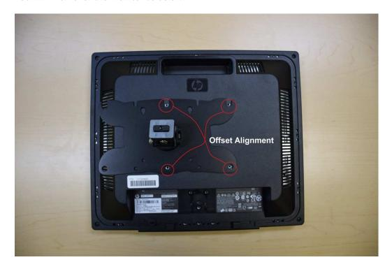
Use the VESA mounting screws provided with your mount to attach the monitor to the bracket. Once the hinge assembly is secured to the monitor, it will be ready for attachment to the monitor mount arms.
