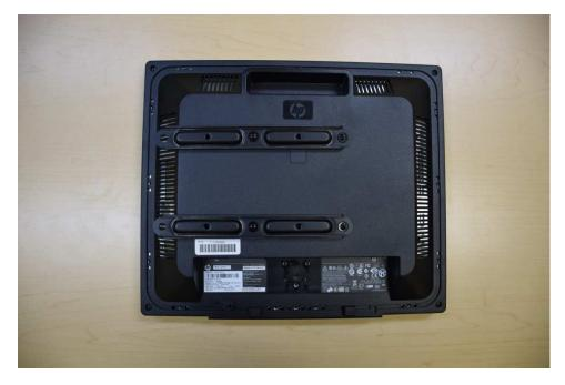
The screws used here should be the VESA mounting screws that come with you monitor mount and not the screws from the AMRV200.
