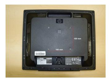
Each of the AMRV100A brackets would be placed over the VESA holes of the monitor as illustrated below.
