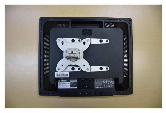
Adjust the position of the VESA hinge to align the pre tapped screw holes and use the VESA screws provided with the Mount to attach the bracket to the hinge. At this stage, all the screws should be tightened to keep everything in place.
