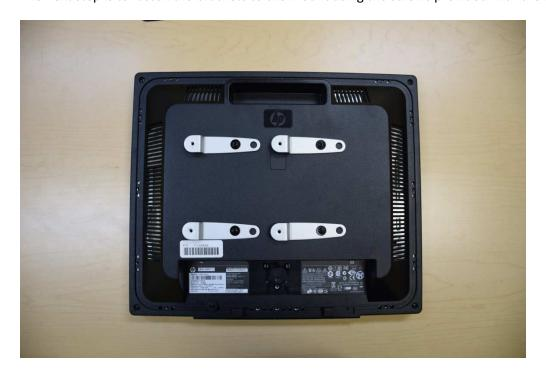
Refrain from tightening the screws. This will keep the brackets movable so that they can be adjusted to fit the VESA hinge bracket. The next step is to match the hinge bracket to the AMRV100A.
