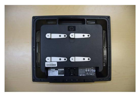
The AMRV100A comes with 2 sets of holes on each bracket. The middle hole is used in this illustration. The outermost hole should be used if a longer offset is desired.
