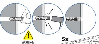
Anchors that are not fully set in solid concrete will not support the applied load resulting in an unstable, unsafe condition which could lead to personal injury and/or property damage. Consult a construction professional if you have any doubt about what this means in regard to your particular situation.
