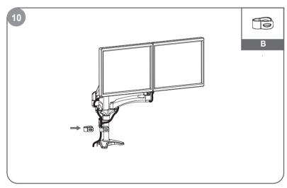
Insert cables into cable covers.
