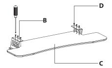
Screw up the six screws through the steel plate to the back of the keyboard tray
