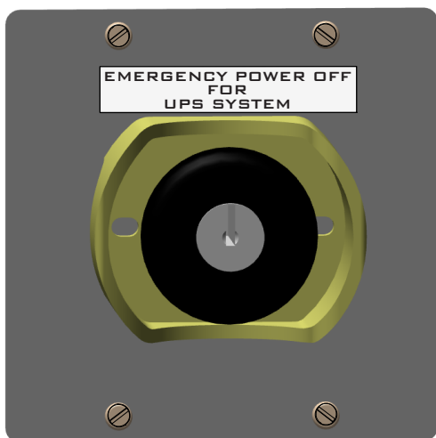
REPO Switch (Front View)
