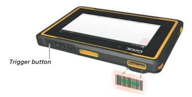
**NOTE:** Improper ambient light and scanning angle can affect the scanning results.
