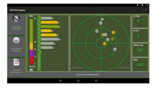
SBAS (satellite-based augmentation system) provides additional accuracy and reliability for the GPS devices. Ground stations are necessary to achieve the purpose. The SBAS feature works where such stations exist. You can enable the SBAS feature. (See "Getac Settings"
