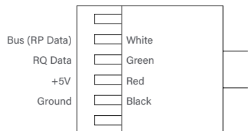
RJ-14 Pin-Outs (Tab Is Facing Down)
