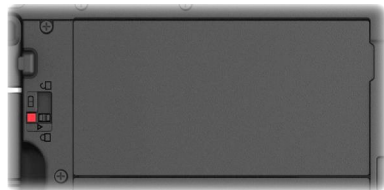
Incorrect (revealing red part)
