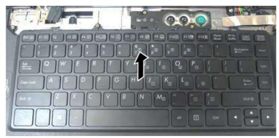
4. Remove four screws (370102010416) lock the keyboard bracket cover, then remove the keyboard bracket cover.
