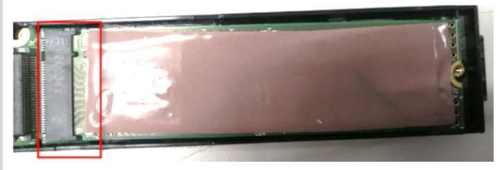
6. Assemble the SSD cover and fix the cover using the one screw (371102010432). **Attention: The hook needs to be clamped tightly.**
