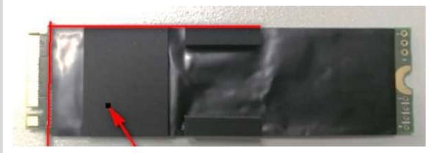
4. Paste the thermal pad onto the other side of the SSD.
