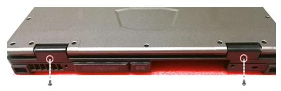
2. Remove seven screws (371102010432) lock the keyboard cover and hinge cover. Then remove the keyboard cover and hinge cover.
