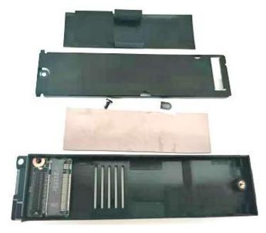
3. Paste the Mylar onto the new SSD.
