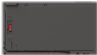
Incorrect (revealing red part)
