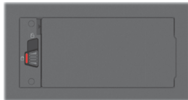
Incorrect (revealing red part)
