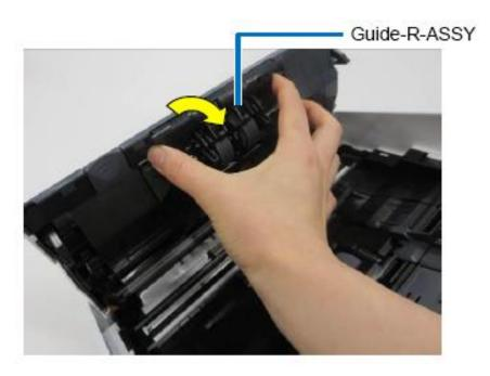
(3) Lift the BR-Roller-ASSY on the right side, remove the right-side shaft (1), and pull out the left-side shaft from the slot (2).
