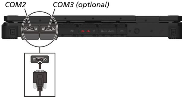
**X600 Pro** has one more serial port (COM3 or COM4) on the expansion unit.
