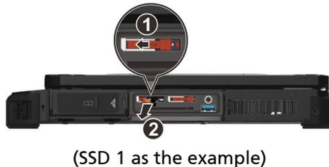
4. Noting the orientation, insert the SSD canister all the way into the slot.
