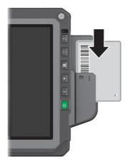
**NOTE:** Make sure to press the magnetic stripe firmly against the reader when swiping the card. A poor contact or an incomplete swipe action will result in an unsuccessful reading.
