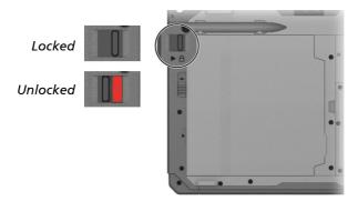
**CAUTION:** Make sure the lock is correctly locked, not revealing the underneath red part.
