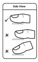
After placing your finger on the scanner, lift it up and place it down again. You should slightly move your finger between each reading. Repeat this action several times (normally between 12 and 16 times) until the fingerprint is enrolled.
