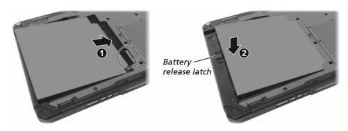
2. Slide the security lock to the locked position (  $\Box$  ).
