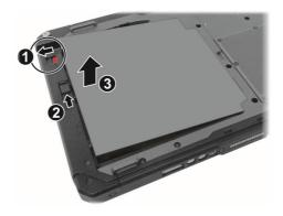
3. Fit another battery pack into place. With the battery pack correctly oriented, attach its connector side to the battery compartment at an angle (①) and then press down the other side (②). The battery release latch should automatically engage.
