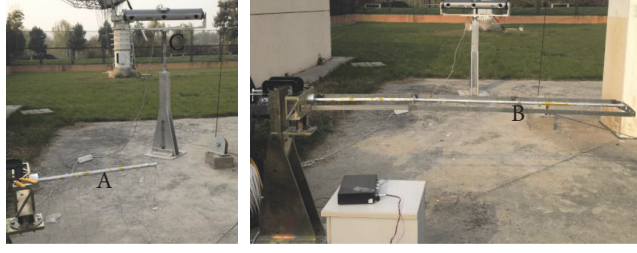
FIGURE 6: Static test setup. The single beam (A), frame structure (B), and NDI Optotrak Certus (C).
