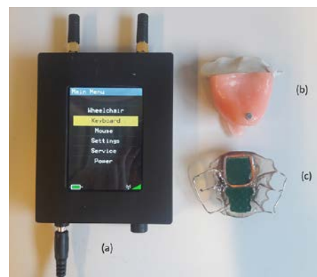
Fig. 1. The inductive tongue control interface modules. a: The central unit, b: The activation unit on a phantom tongue, c: The mouthpiece
