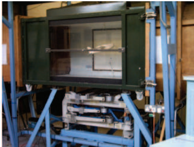
Fig. 1. The flexible suspension system for wind tunnel
