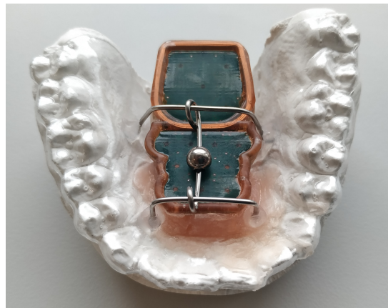
Fig. 3: Noninvasive tongue-computer interface.
