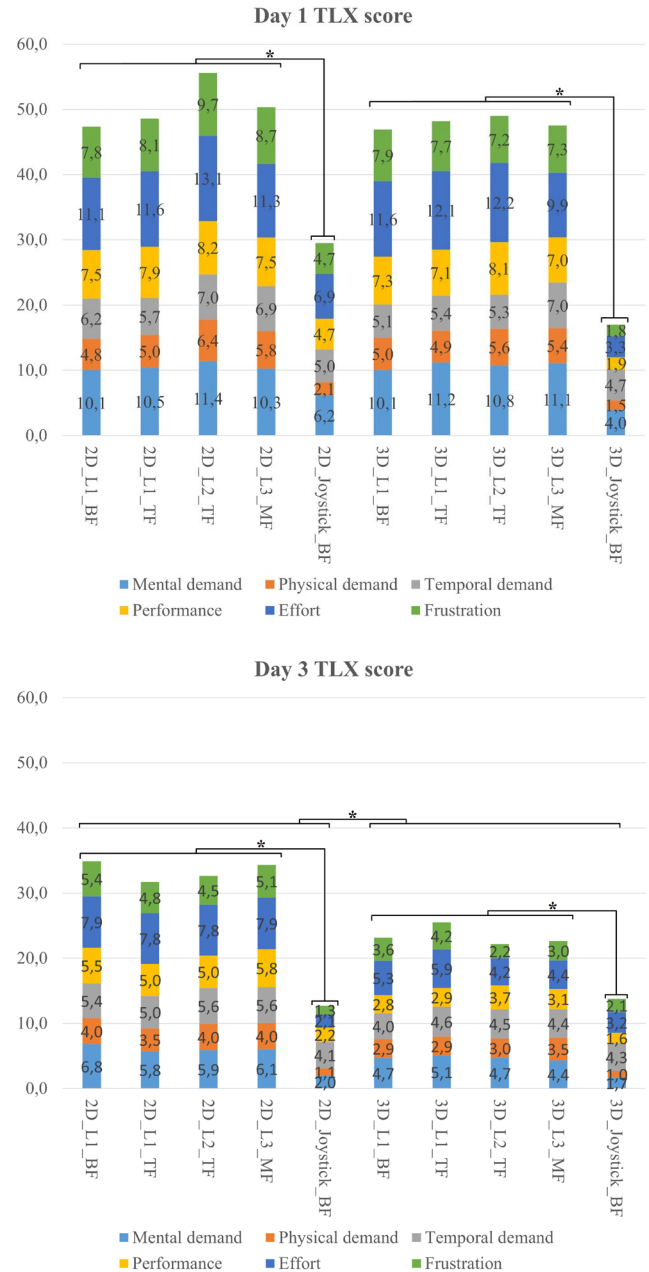
Fig. 11. NASA-TLX questionnaire results from Day 1 and 3. L1_BF was presented in [29] and implemented for control in base-frame and tool-frame (L1_BF and L1_TF). L2_TF is the new improved layout for control in tool-frame where a "GO" button and a dedicated button for mode switching were introduced. L3_MF was adjusted for control in BF. In order to maintain control of all of the available DOF's, two DOF's were introduced as toggle buttons (forward/backward and roll+/roll-). Joystick_BF represents control with the standard joystick that comes with the JACO ARM. The * indicates a significant difference.
