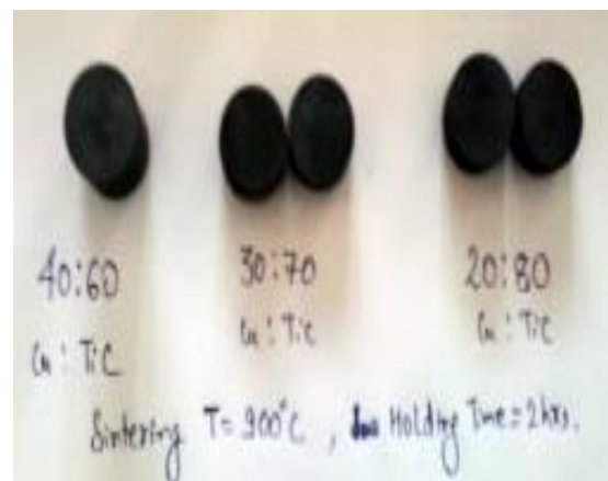
Fig5.2: Top view of compacted tool
