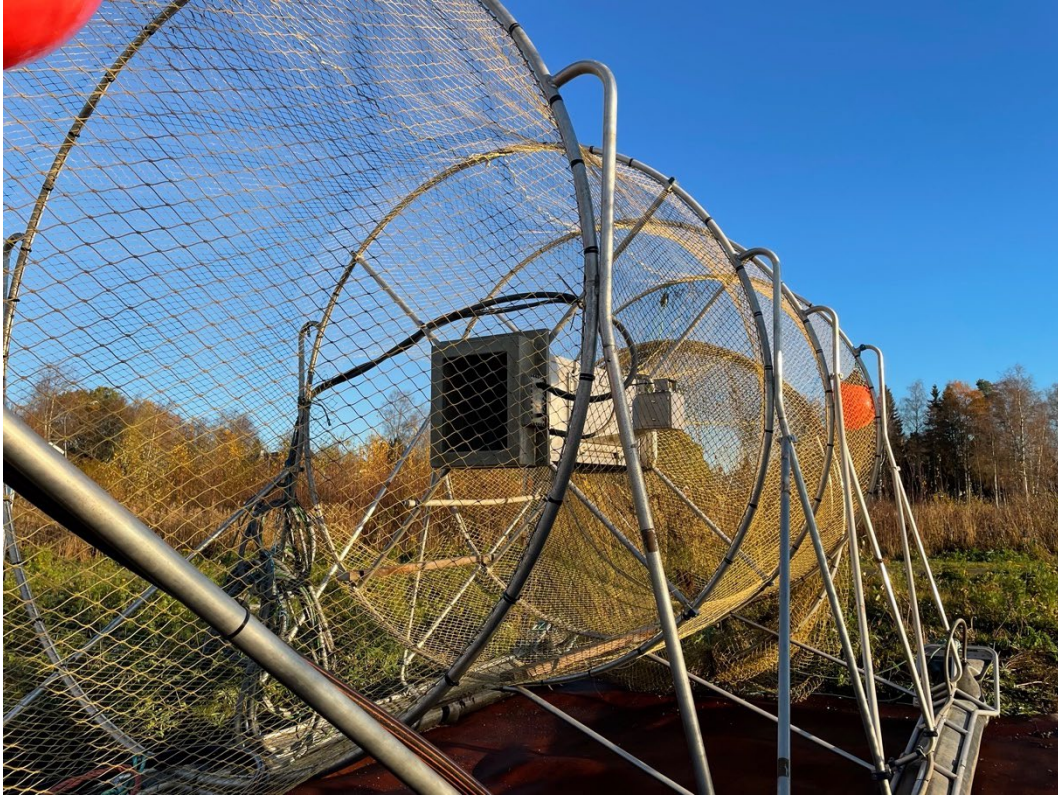
Figure 2. The camera tunnel inside of the trap.
