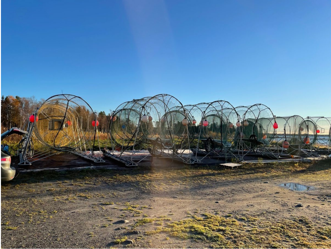
Figure 1. The traps used to catch salmon. The yellow one furthest to the left has the camera mounted in the center.
