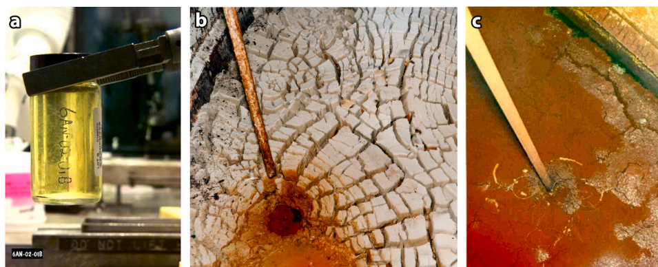
Fig. 2. Photographs of (a) supernatant in a laboratory sample, (b) saltcake, and (c) sludge taken inside of a tank.
