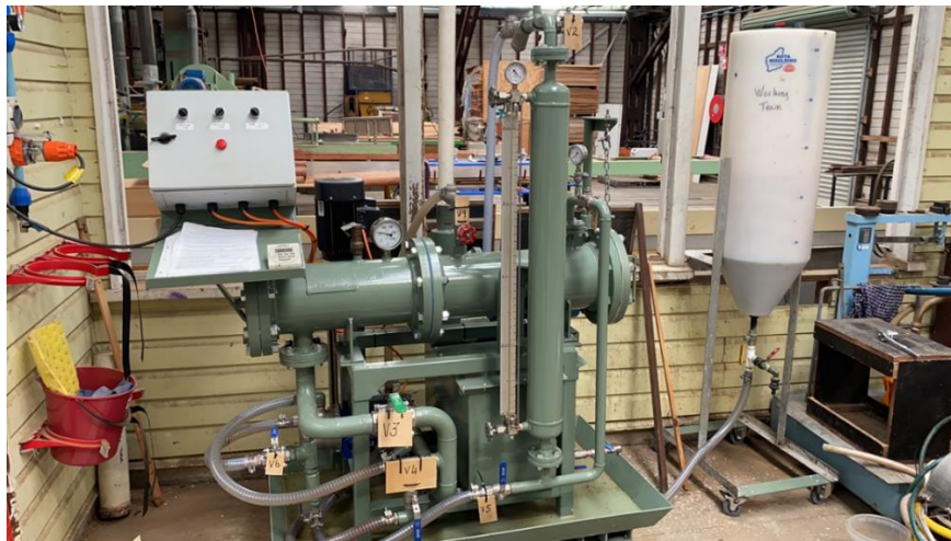
Figure 2. Vacuum-impregnation chamber for wetting experiments at the Salisbury Research Facility
