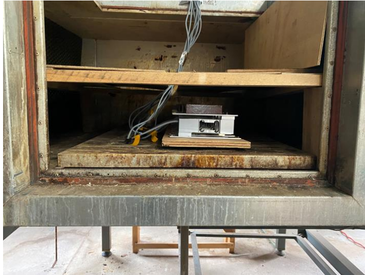
Figure 6. 1D SPG sawn timber drying test setup
