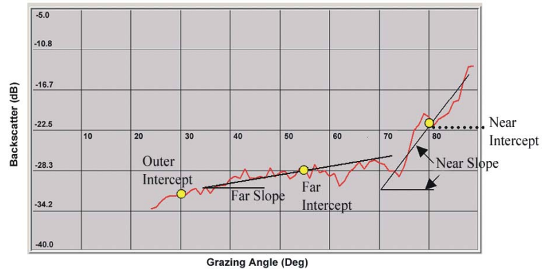
Figure 3. Stacked backscatter angular response measured by a Simrad EM3000 multibeam sonar, with some of the AVO parameters.
