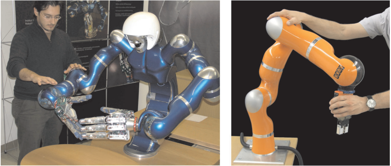
Fig. 1. Physical cooperation between humans and robots is desirable for future robotic applications and poses the fundamental question of how to ensure safety for the human during such scenarios. As an example a human is interacting with the DLR humanoid Justin (left) and the KUKA Lightweight Robot (right). The KUKA Lightweight Robot is based on the DLR-Lightweight Robot III (LWRIII) and is the result of a technology transfer from DLR to the robot manufacturer KUKA.
