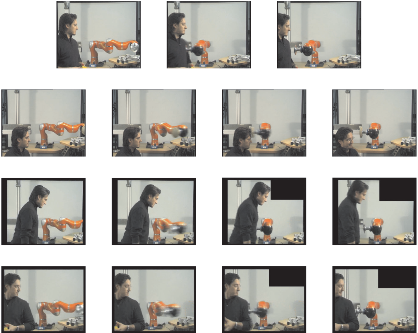
Fig. 9. Impact tests with a human chest at 2.7 \text{ m s}^{-1} and head at 1.5 \text{ m s}^{-1} . The impact velocities for the abdomen and the shoulder were also 2.7 \text{ m s}^{-1} which is the maximum velocity of the robot. During all of these experiments the robot does not react to the activated collision detection. The robot stopped only when the maximum nominal joint torques were exceeded. However, as a result of the crash test dummy experiments, the impact forces caused by the very short collision duration cannot be affected by this feature due to its delayed reaction. These tests were initially described in Haddadin et al. (2007a) and support, if not even prove, the conclusions stated previously.
