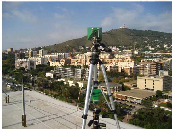
Fig. 8. Interferometric antennas and scene on the background for the backscattering geometry.
