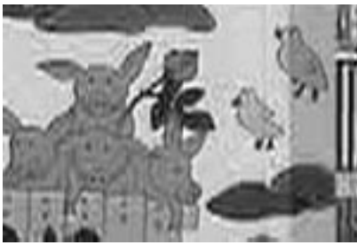
Fig. 11. Direct progressive SDTV. Mobcal at 5 Mbs/s. Part of the I-picture (frame 24, top field). PSNR = 28.5 dB.
