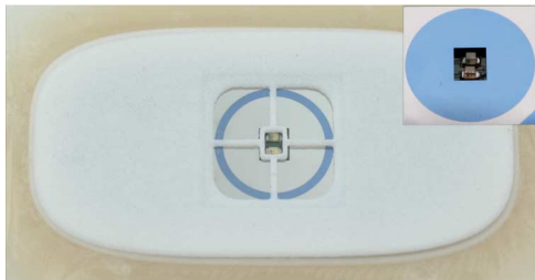
Fig. 7. The photo shows an E-type photodiode packaged and assembled into a patch. The two LEDs are seen in the center. The chip in the upper right corner shows a F-type photodiode with a micro-structured surface for better absorption of light.
