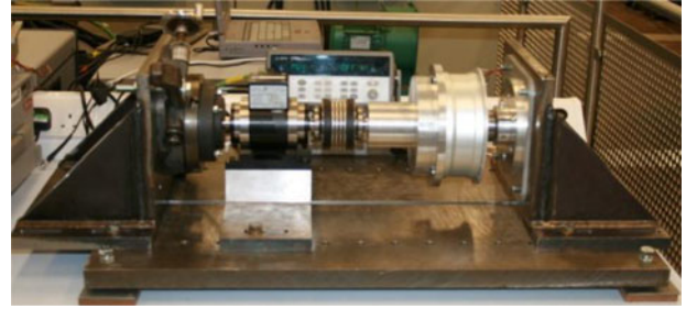
Fig. 16. Test setup showing the combined-phase machine connected through an in-line torque transducer to a rotary dividing head.
