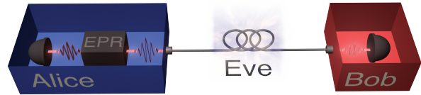
FIG. 1: Conceptual picture of a 1sDI-CVQKD protocol. From the perspective of Alice (Bob) the local devices are known and allow a secret key to be extracted from a direct (reverse) reconciliation protocol, even though the other party exists only as an unknown red (blue) box.
