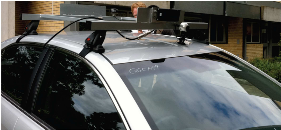
Figure 2: Instrumented Toyota Camry vehicle with IBEO laser, GPS, OBD-II reader, accelerometer (Vigil) and video cameras
