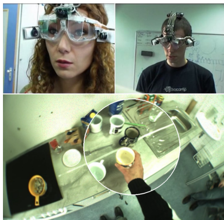
Figure 7: A gaze directed camera used in [111]; the camera itself is shown in the upper images. The lower image shows a superimposed camera view generated by the device (reprinted).
