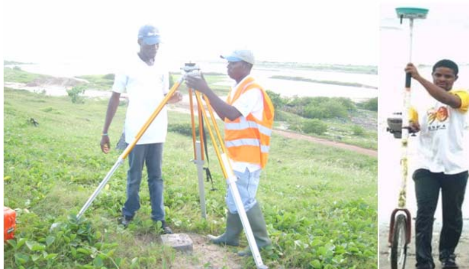
Figure 4. Kinematic GPS survey using a monocycle mounted with GPS receiver.
