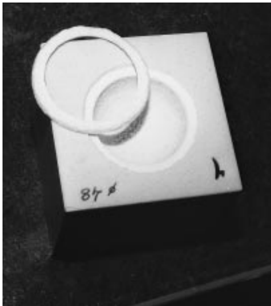
Fig. 7 Annulus of foam removed by cup rim at pull-out and lever-out
