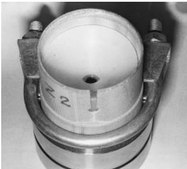
Fig. 2 GFRE tube mounted on a holder and cavity base support
