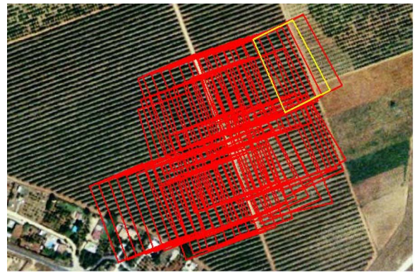
Fig. 9. Footprints for the images acquired during a flight plan conducted over an orange orchard. Red rectangles correspond to single image frames. The yellow rectangle represents the overlapping of two consecutive images (stereo-pair).
