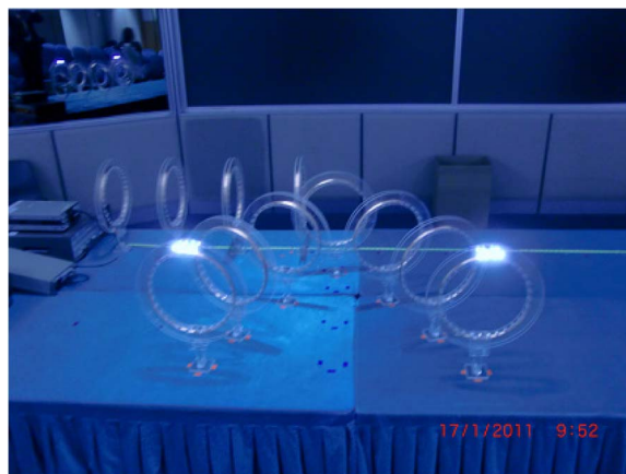
Fig. 14. Use of Tesla’s loop resonators in a domino form for wireless power transfer. (The power flow path is bent and then split into two branches for powering two LED loads.)
