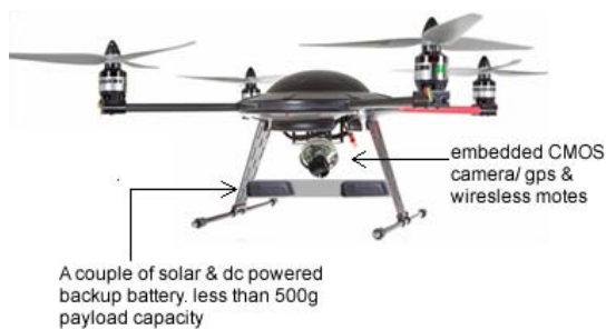
Figure 2. A quadcopter with a payload of solar charged batteries to increase flight time.
