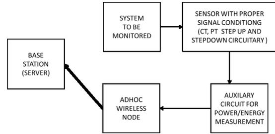
Fig1. System architecture for the power monitoring system
