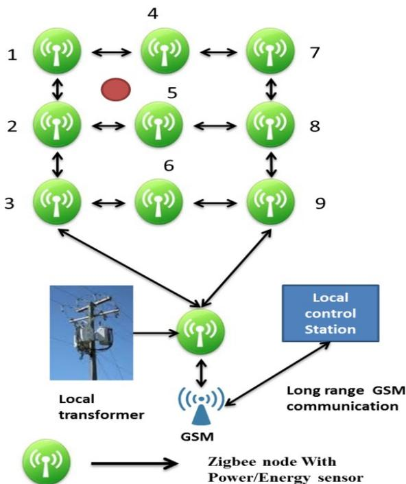
Fig 9. Proposed theft detection algorithm model
