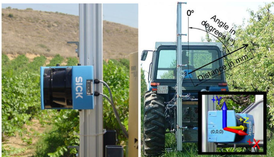
Fig. 1 LMS-200 scanner ( left ) and mounting used in the field trials ( right ) (Rosell et al. 2009b)
