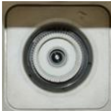
Figure 2. Photograph of the single PICS injector, from aft-looking-forward view.
