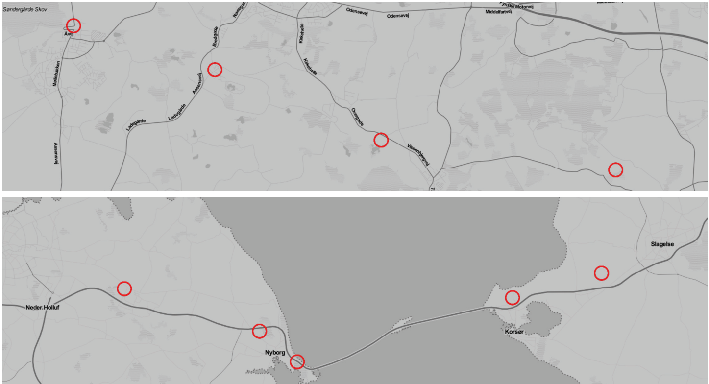
Fig 9. Two examples of stop-locations found using WiFi data which are not geographically stationary. Each plot shows one stop location inferred from WiFi data, each circle shows a single GPS estimation associated with the location. The two stop-locations are most likely based on access points which are present in a train or a bus.
