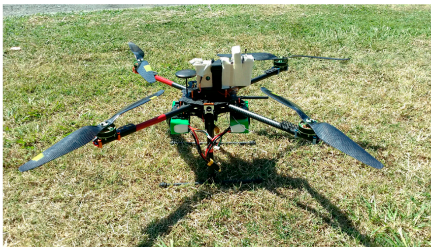
Figure 5. Quadcopter and modular gas-sensor system integrated.
