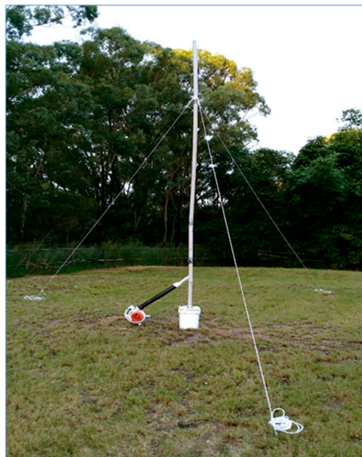
Figure 14. Powder ejection system setup.
