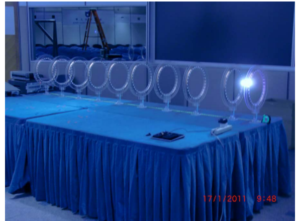
Fig. 16. Straight coaxial domino chain of 3 m and a load of four 8-W LEDs ( d_{\text{total}}/r ratio = 19.4).
